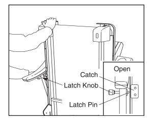
2. Hold the metal frame firmly with both hands, and lower the treadmill to the floor. CAUTION: To decrease the possibility of injury, do not lower the treadmill by gripping only the plastic foot rails. Do not drop the treadmill frame to the floor. Be sure to bend your legs and keep your back straight.
